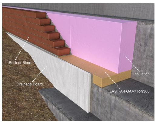
LAST-A-F0AM® R-9300 reduces thermal transfer between the building insulation envelope and the soil. These structural insulating blocks have a high-compressive strength necessary to support the load of the brick or block wall. It will not rot or decompose in below grade applications, and does not retain moisture so it can be left exposed to the elements during construction. The R-9300 is also chemically compatible with most grouts and concretes used.
