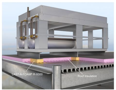
LAST-A-F0AM® R-9300 structural thermal blocks have a high compressive strength that can withstand heavy weight loads for the life of the equipment it is supporting. The R-9300 blocks are chemically inert and will not react with metal or single-ply roofing systems. The blocks do not absorb moisture and can be left exposed to the elements during the construction process.
